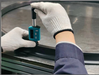
Metal rings hardness test (Rockwell hardness tester)
