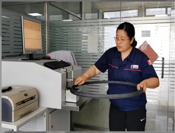
Material content analyzer (The spectrometer for metal Mo Cr Fe analysis)
